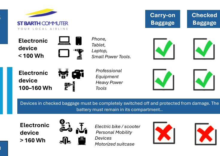
Calculation of a battery's energy: Wh = V × Ah
